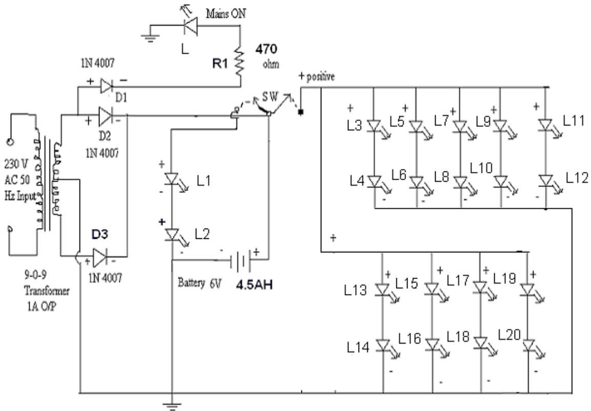
Figure 3.7: torch using series and parallel connection
