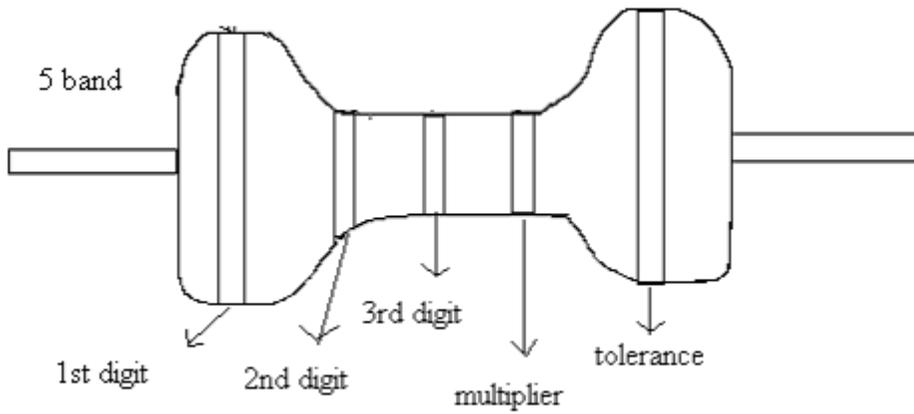
Figure: - 2.6 photo of resistor {{ Show actual photo of resistor)
