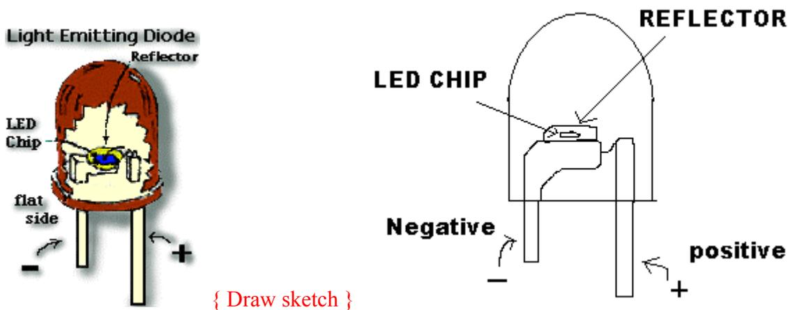
Figure: - Light Emitting Diode (LED)
