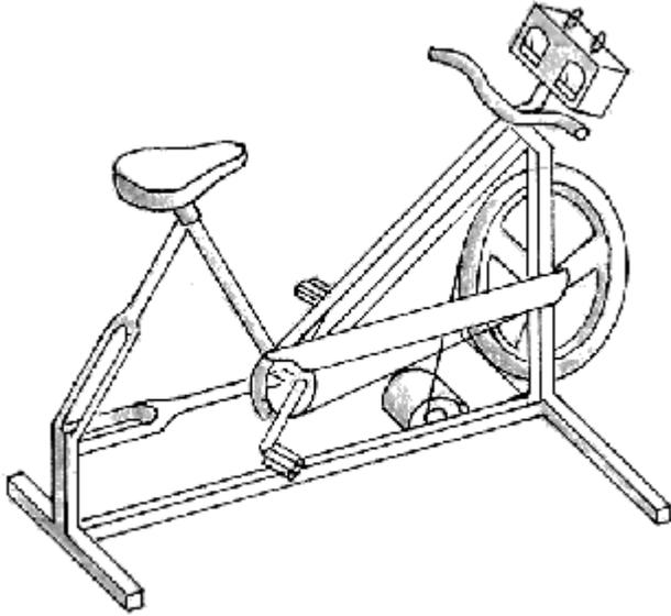
Figure 4.3: - pedal power generator
