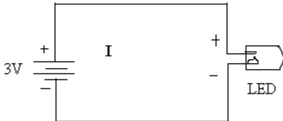
Figure 2.14: - LED connect on battery
