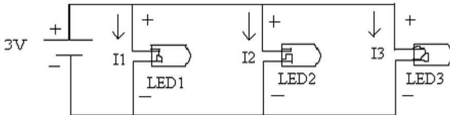
Figure 2.16: - increase current capacity
