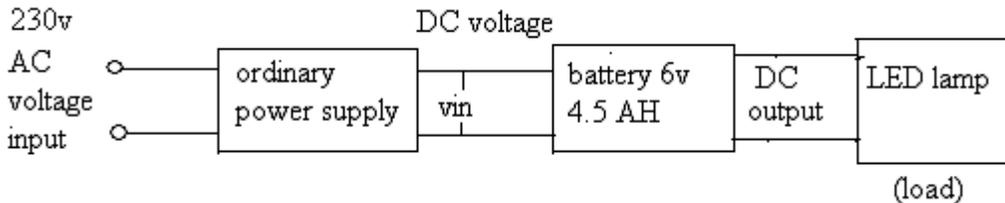
Figure 4.1: - Battery charge using grid power
