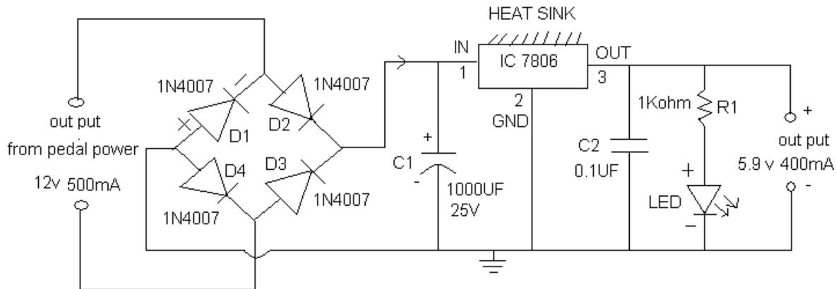
Figure: - mobile charger using pedal power
