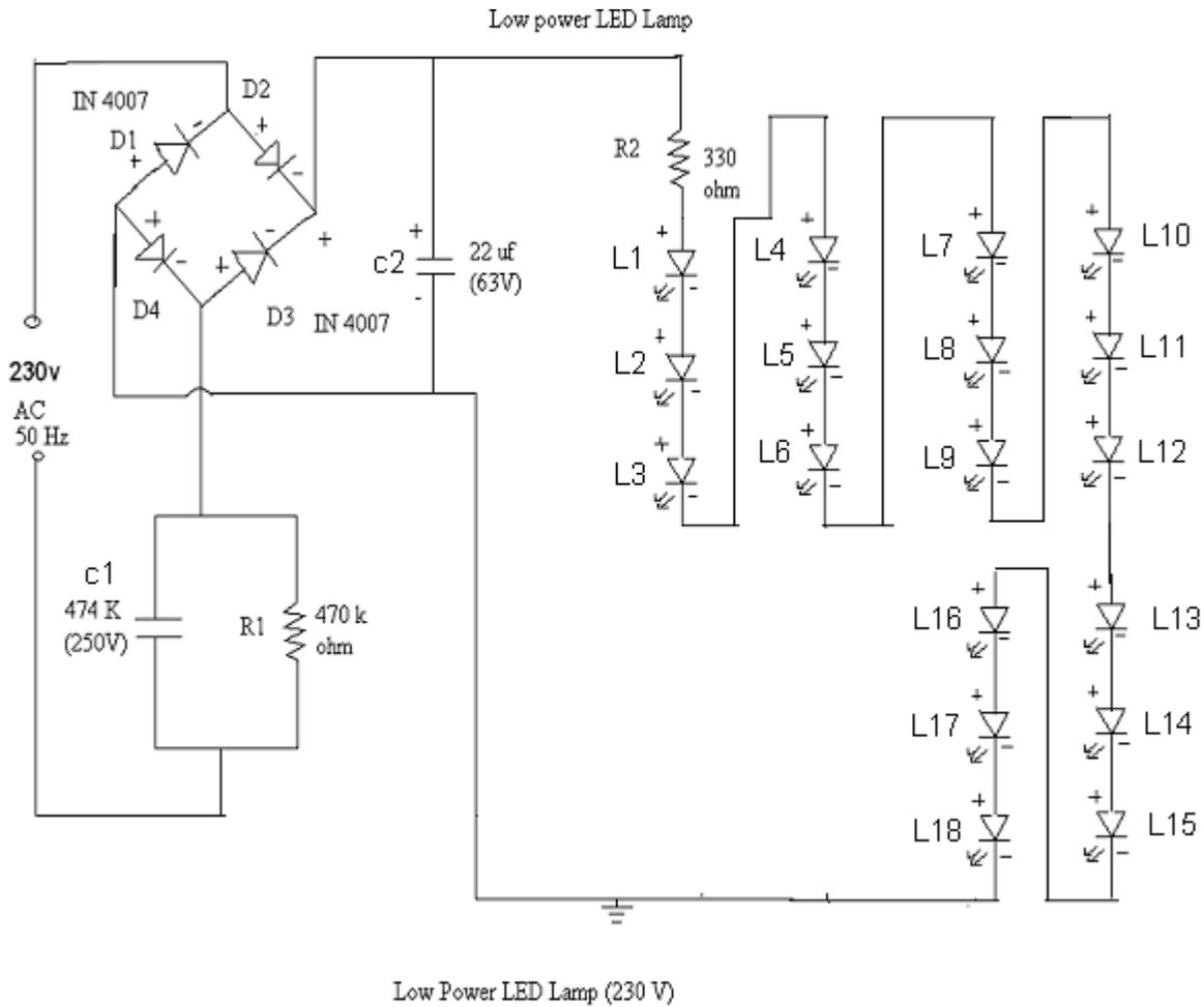
Figure 3.2: low power LED lamp operate 230v.
