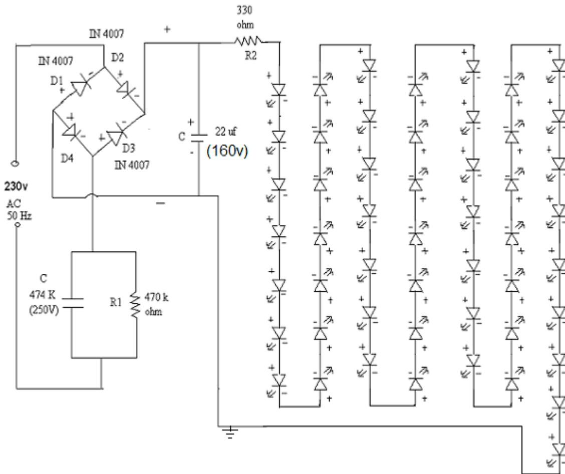
Figure 3.9:- LED strip operate on 230 volt.
