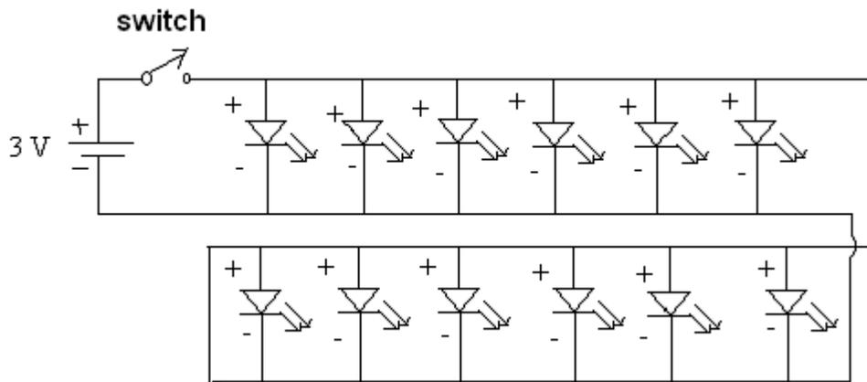
Figure : parallel connection for torch
