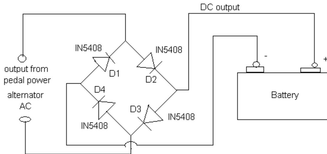
Figure: 4.6 connection for pedal power
