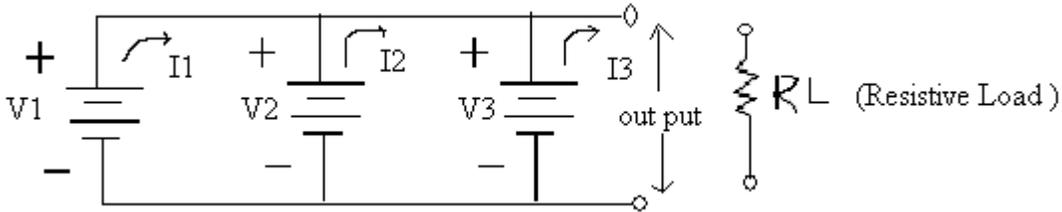
Figure 2.13: - battery connect in parallel form
