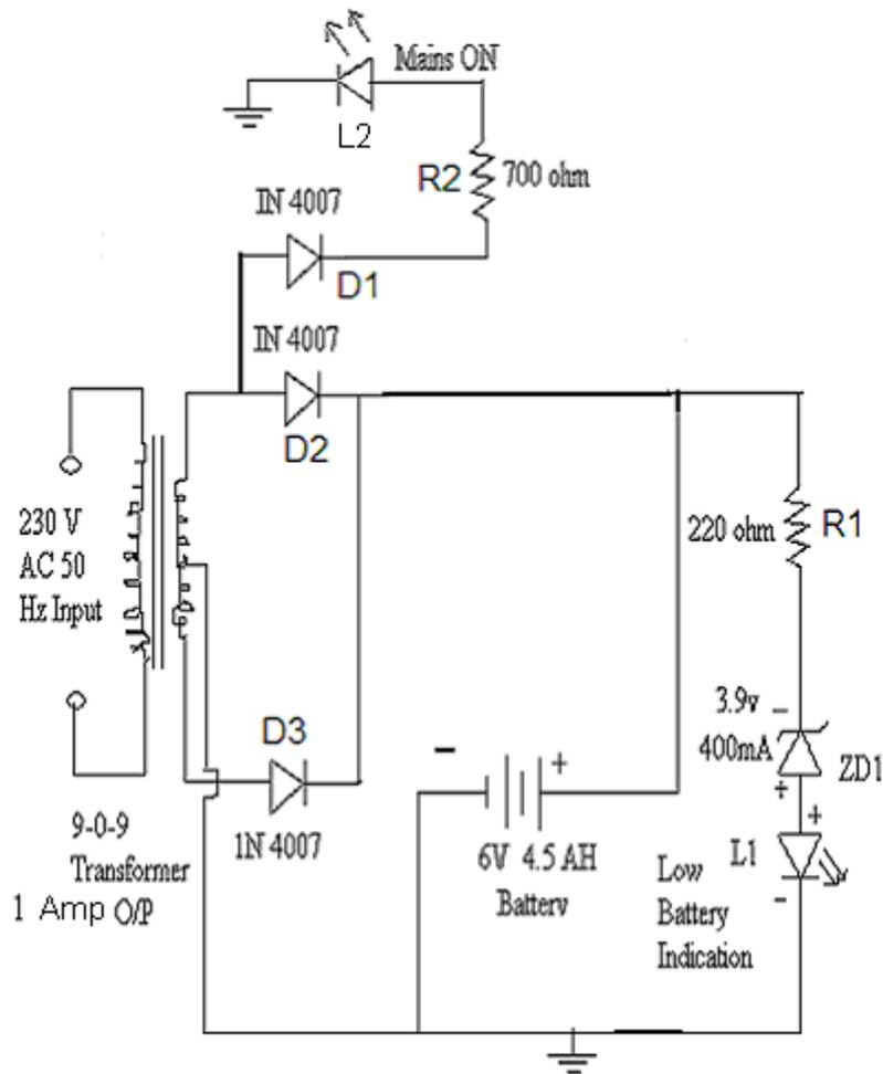
Figure 4.4:- battery charger for 6v battery.
