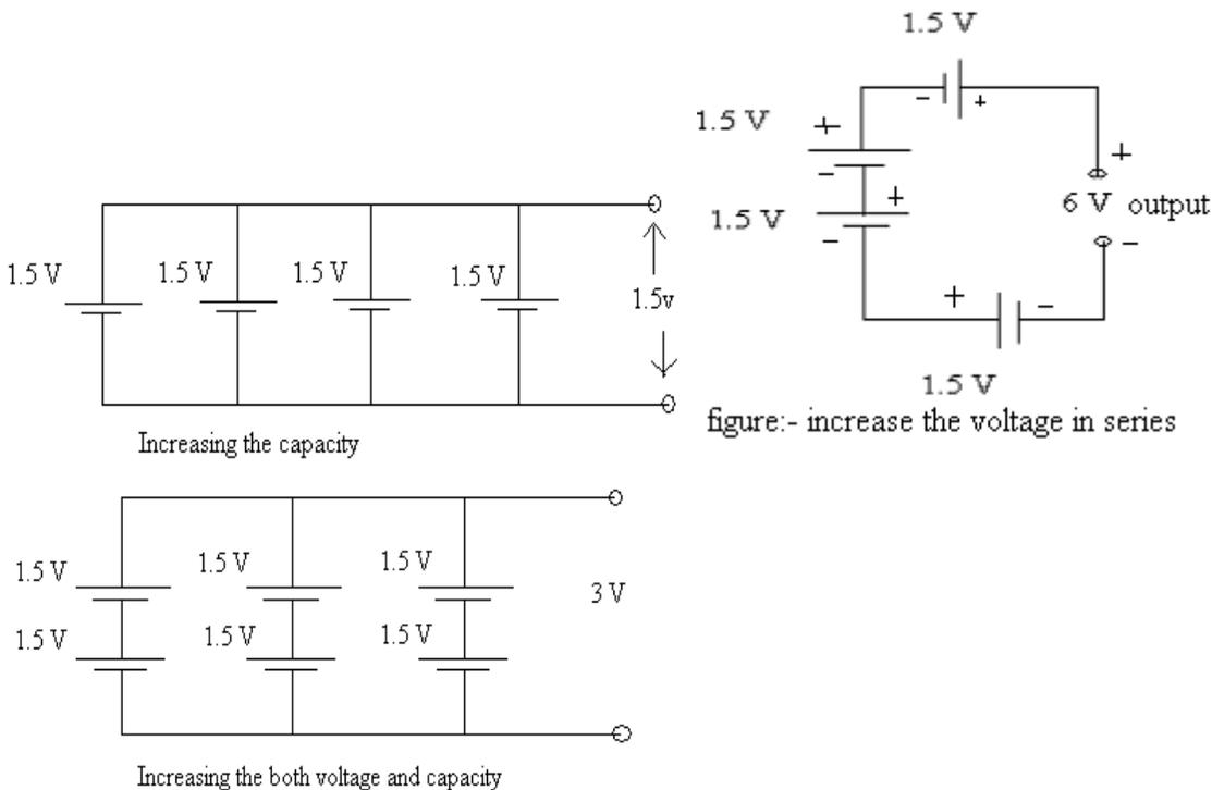
Figure 6.1 battery connect in series and parallel
