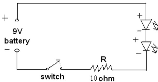
Figure 3.8 :- torch using 9v battery
