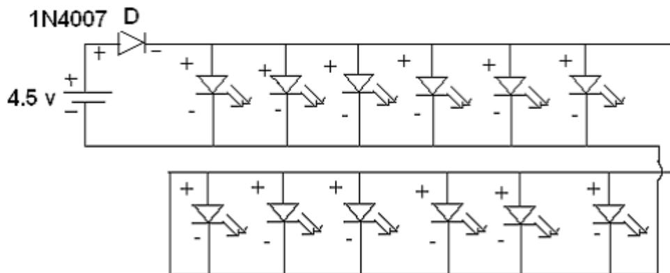
Figure 3.6: parallel connection for torch
