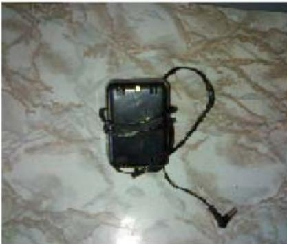
Circuit : Input 230V AC, to charge 6V battery
