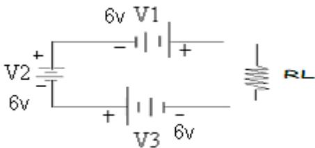
Figure2.12: - battery connect in series
