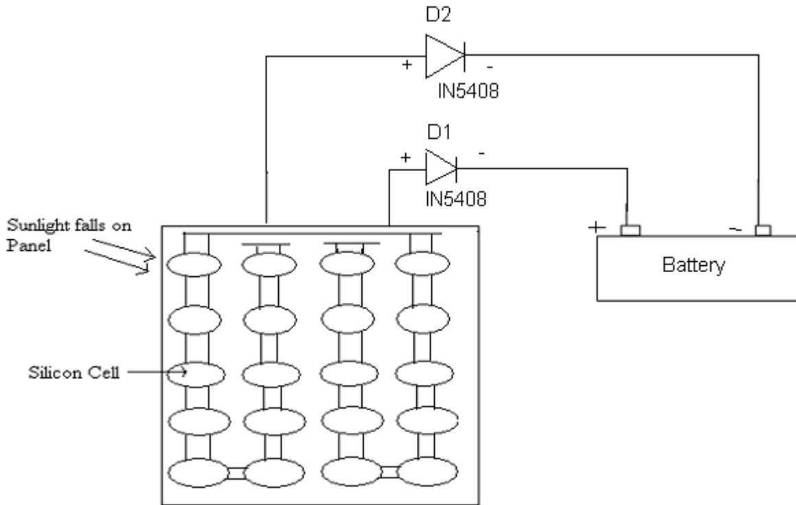
Figure: 4.5 connection for solar panel
