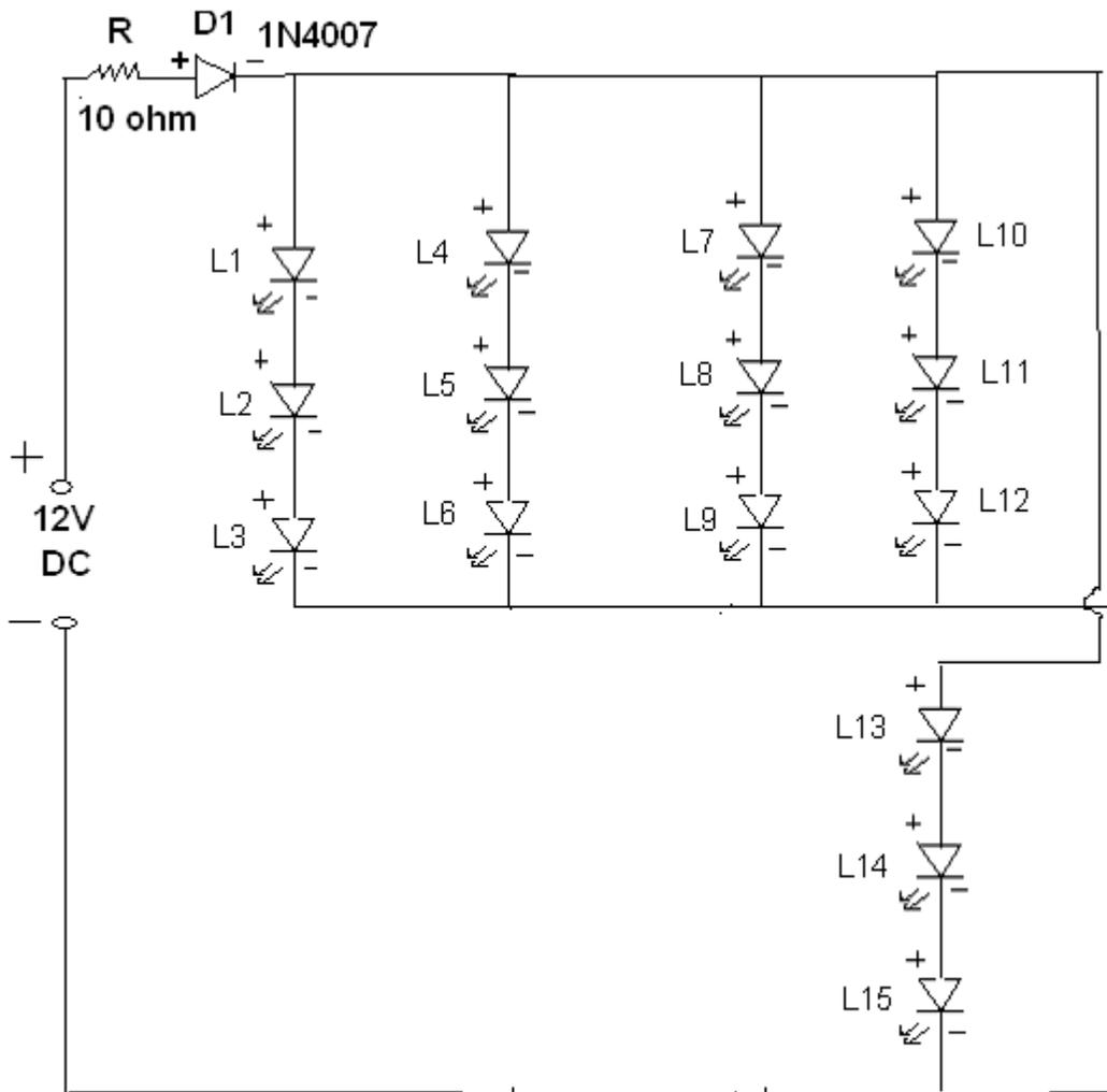
Figure 3.3: DC lamp operate 12v
