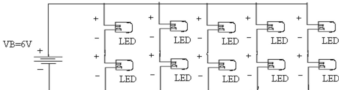
Figure 2.17 LED connect in series and parallel combination
