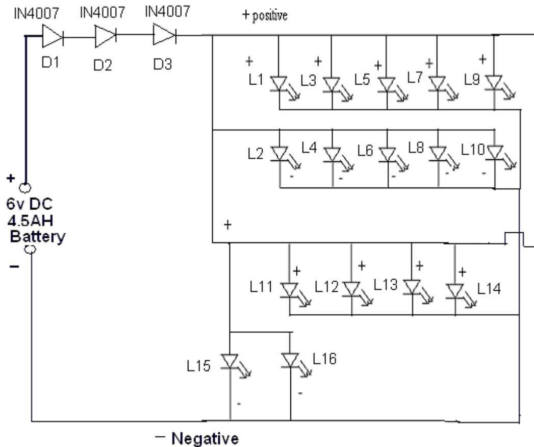
Figure 3.4:- DC lamp operate on 6v battery
